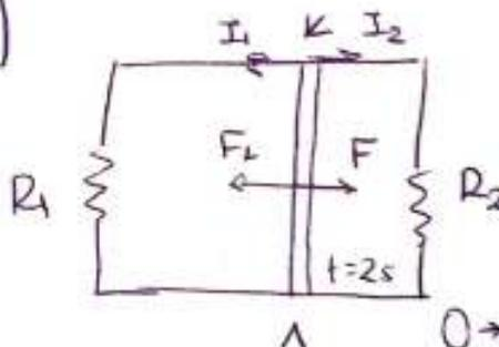
$$R_{1,2} = \frac{R_1 R_2}{R_1 + R_2} = \frac{6 \cdot 3}{9} = 2 \Omega$$
